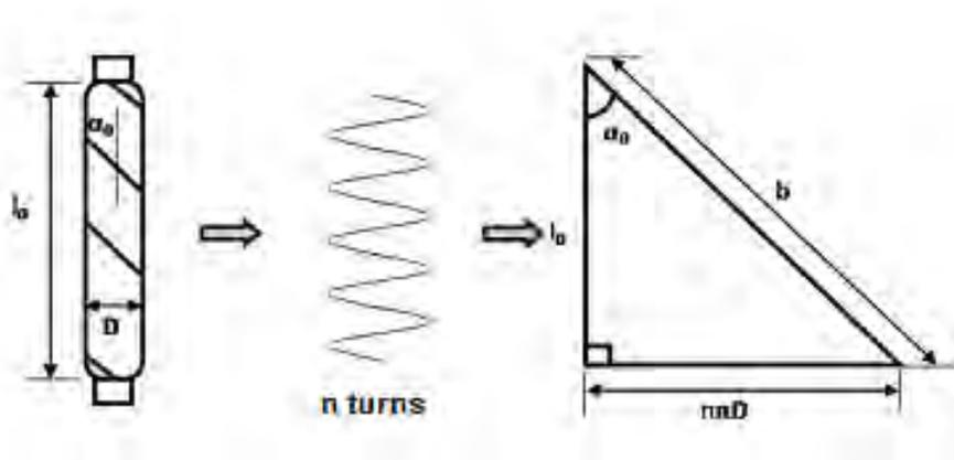
Figure 2. Geometric parameters of the pneumatic artificial muscle
