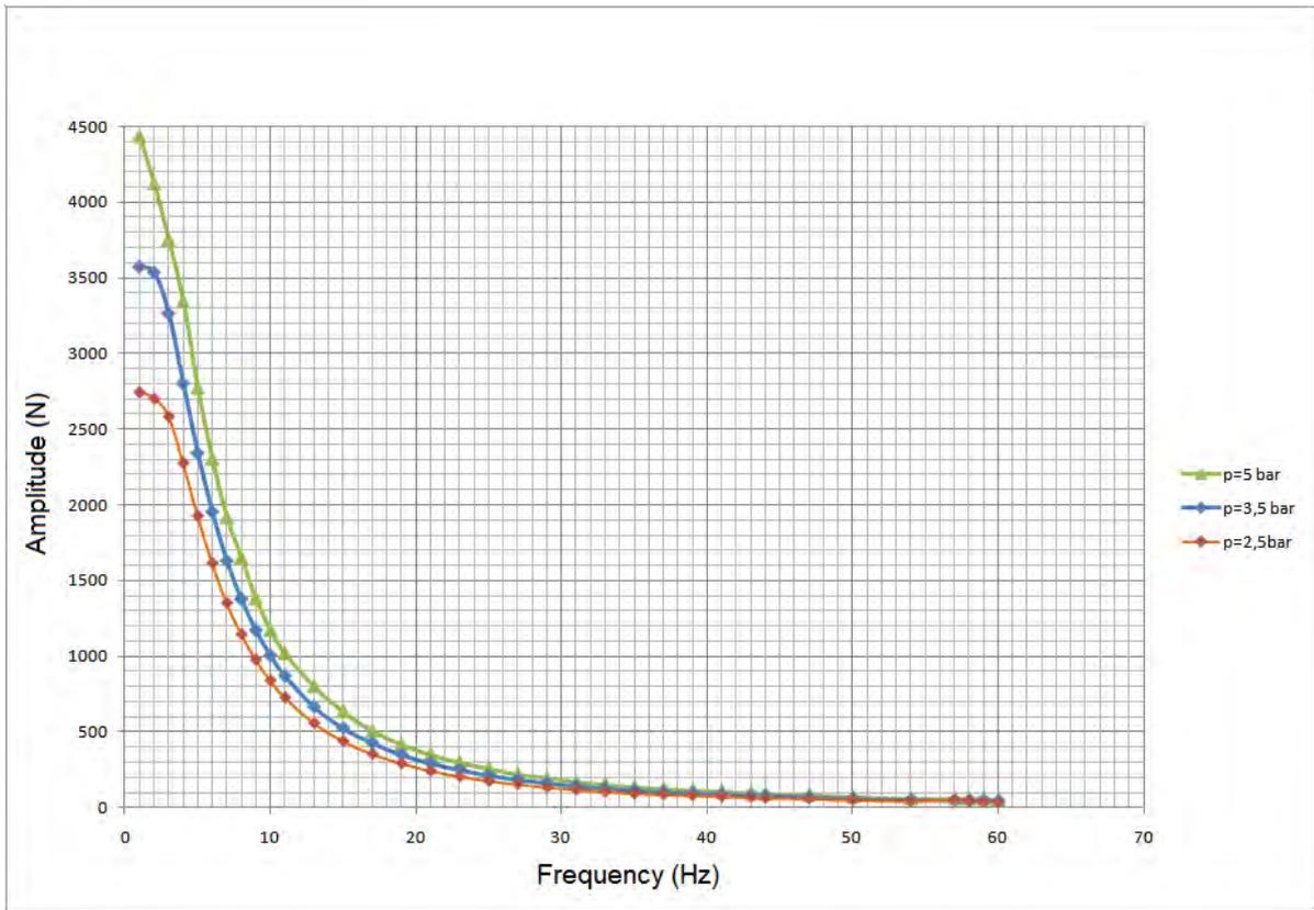
Figure 9. Frequency response of the pneumatic system
