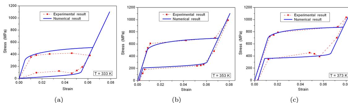
Figure 2: Comparison between numerical results provided by the model (considering TRIP phenomenon) and experimental results by [20] for pseudoelastic behavior for three different temperatures. (a)  $T = 333$  K; (b)  $T = 353$  K and (c)  $T = 373$  K.
