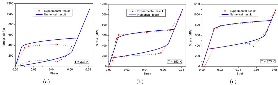
Figure 1: Comparison between numerical results provided by the model (without considering TRIP phenomenon) and experimental results by [20] for pseudoelastic behavior for three different temperatures. (a)  $T = 333$  K; (b)  $T = 353$  K and (c)  $T = 373$  K.
