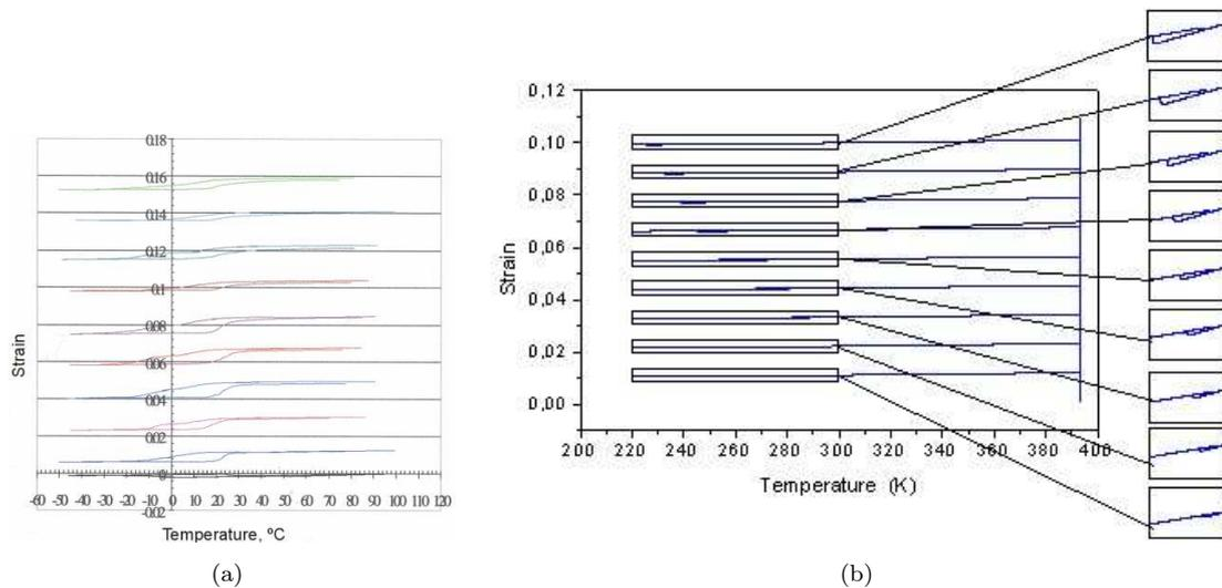
Figure 6: Strain-temperature diagram for qualitative comparison between numerical results provided by the model and experimental results by [24] for cyclic test to verify plastic-phase transformation coupling. (a) Experimental result; (b) Numerical result.
