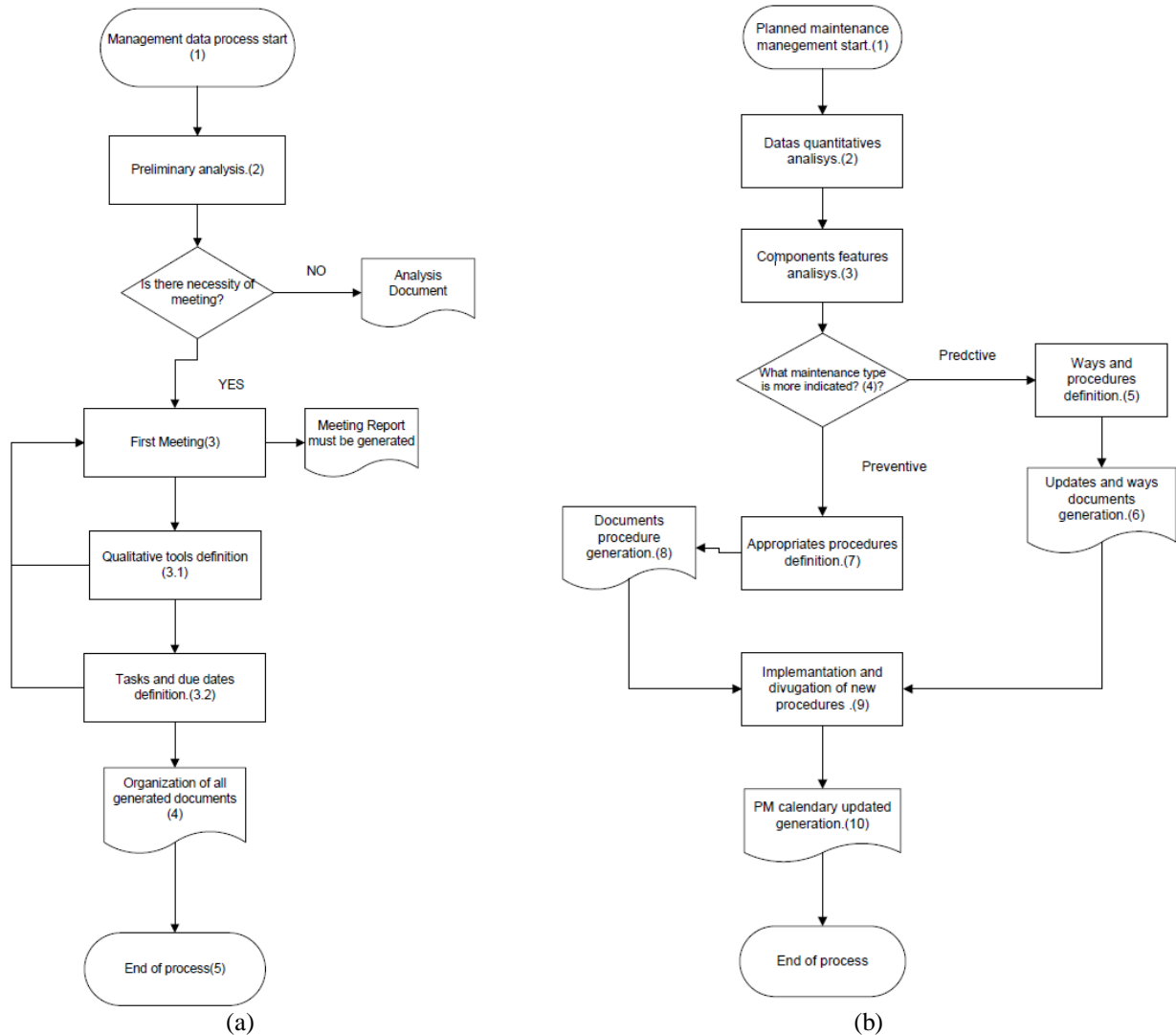
Figure 3 ó (a) Flowchart of data management; (b) Flowchart of planned maintenance management
