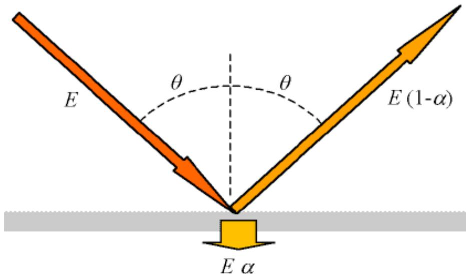
Figure 3. Representation of specular reflection (Tenenbaum and Camilo, 2004)
