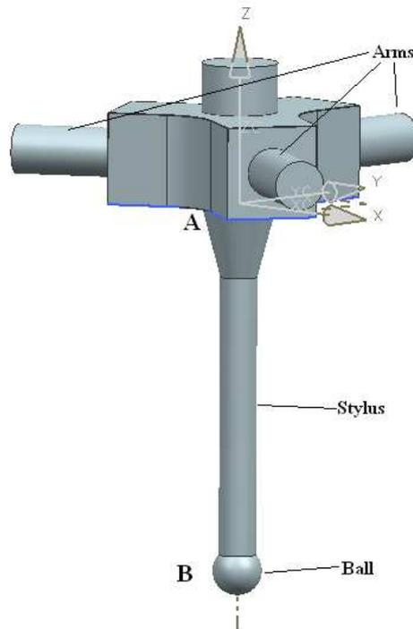
Figure 1. The simplified model of Kinematic contact probe system
