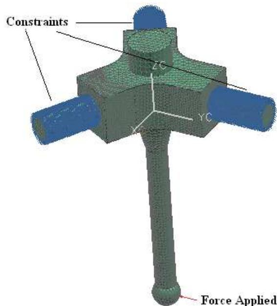
Figure 3. Mesh, load and constraint of the model
