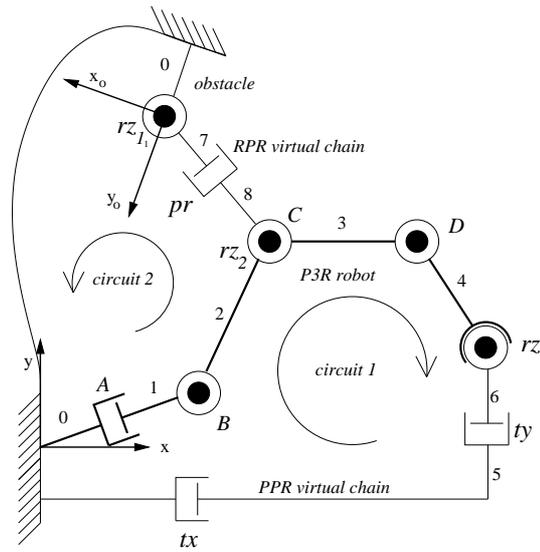
Figure 2.  $P3R$  redundant robot with the virtual chains attached.
