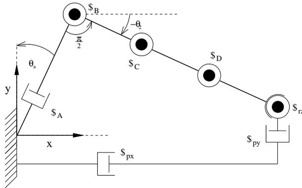
Figure 3. Singular condition for  $P3R$  redundant robot.
