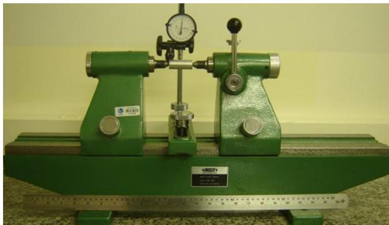
Figure 2. Dial gauge attached to a tailstock device.
