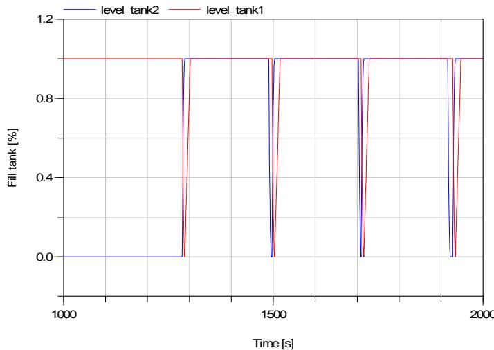
Figure 7. Level tanks in function of time with a heat supply rate of 3170W.
