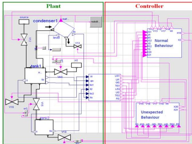
Figure 4. Schematic representation of the system, using Dymola software and Modelica modelling language.
