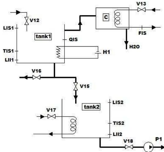
Figure 2. Scheme of the entire evaporator system
