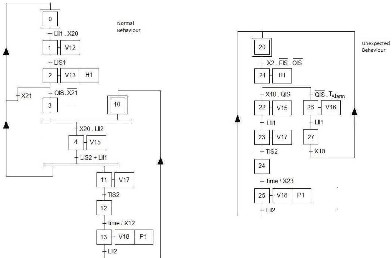
Figure 3. SFC controller specification: normal and unexpected behavior modes.
