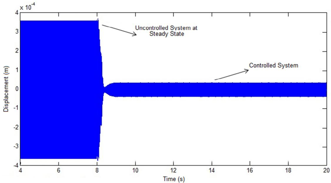
Figure 12. Displacement Signal for the Roller Bearing Position rotor speed of 9930 RPM (Controller with 5 membership functions – 7<sup>th</sup> Simulation)
