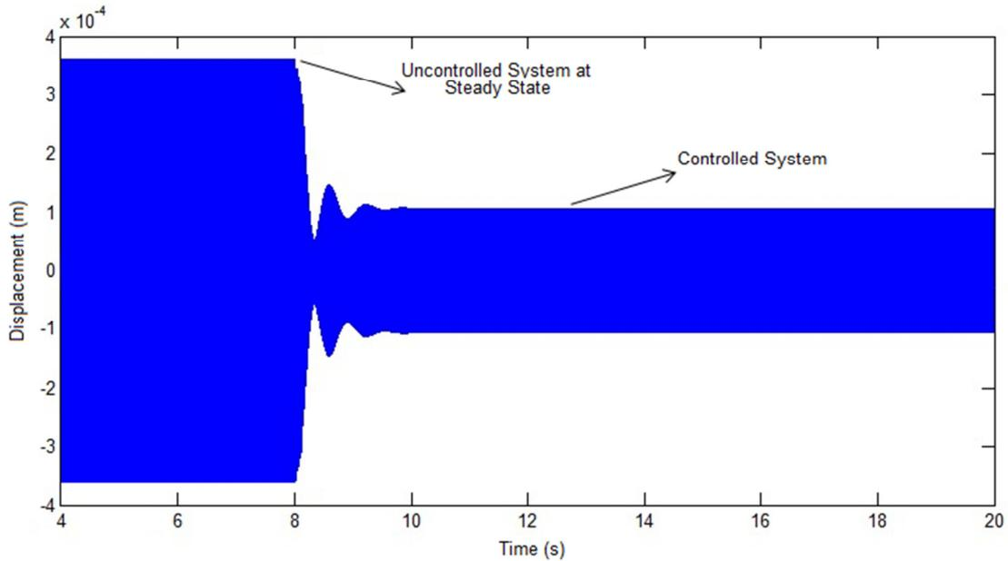
Figure 10. Displacement Signal for the Roller Bearing Position for a rotor speed of 9930 RPM (Controller with 3 membership functions – 4<sup>th</sup> Simulation)
