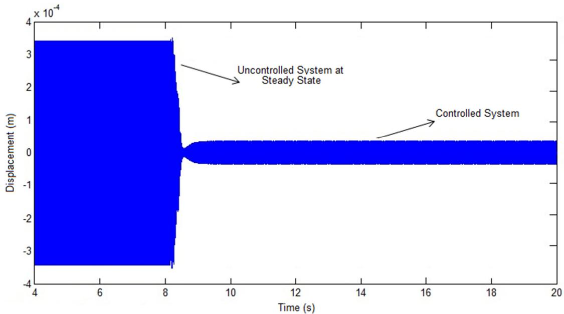
Figure 13. Displacement Signal for the AMB Position rotor speed of 9930 RPM (Controller with 5 membership functions – 7<sup>th</sup> Simulation)
