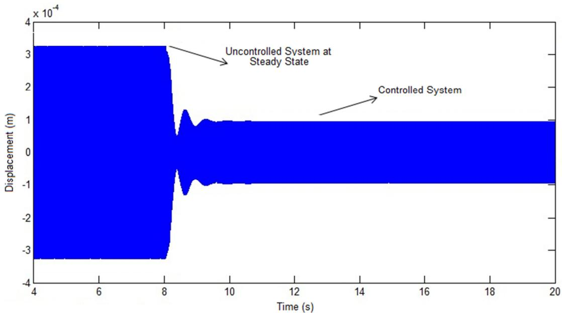
Figure 11. Displacement Signal for the AMB Position rotor speed of 9930 RPM (Controller with 3 membership functions – 4<sup>th</sup> Simulation)
