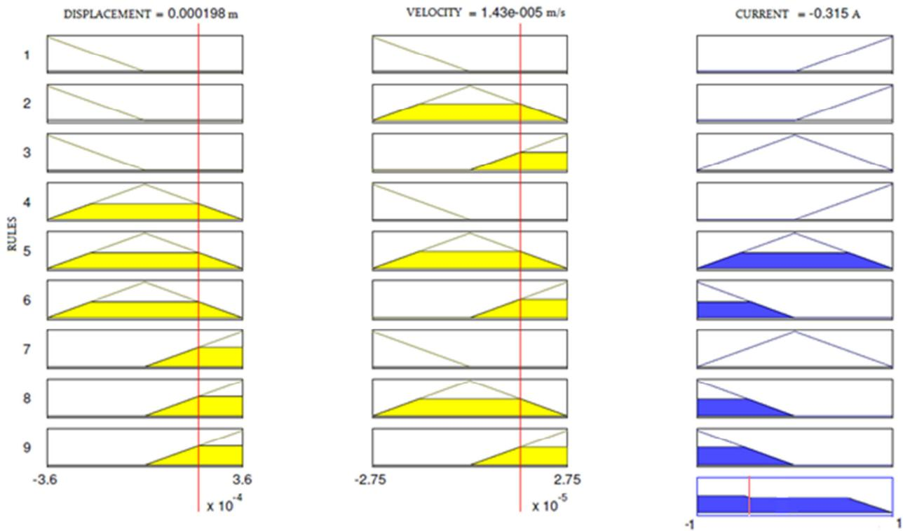
Figure 8. Defuzzification result for an example of a base of rules with 9 rules.
