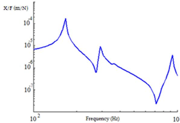
Figure 6. A Bode plot between a force input at the AMB position and the displacement of the rotor at one of the roller bearing positions
