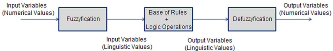
Figure 5. Basic Configuration of a Fuzzy Controller
