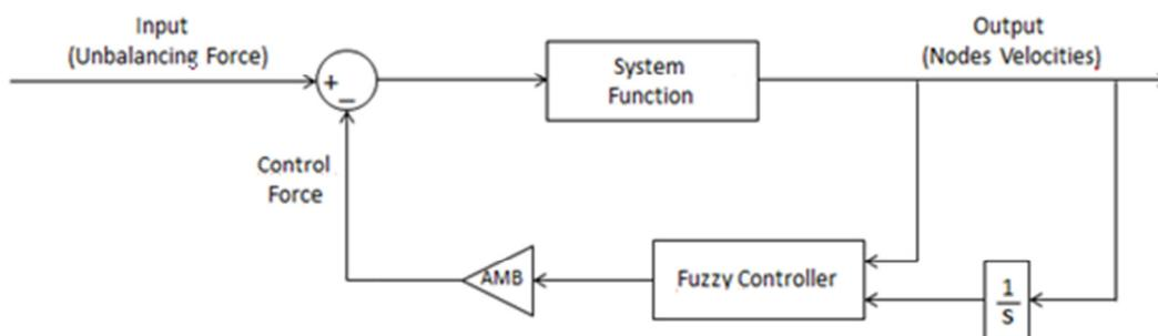
Figure 9. Closed-loop control for the rotor system
