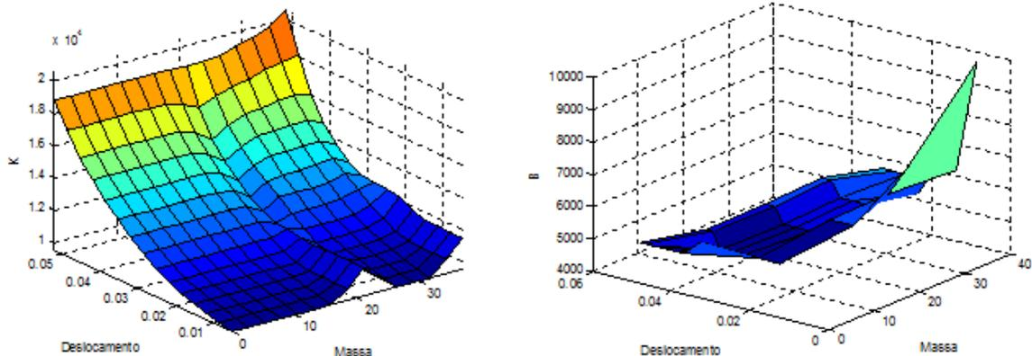
Figure 7. Fuzzy stiffness (left) and damping (right)
