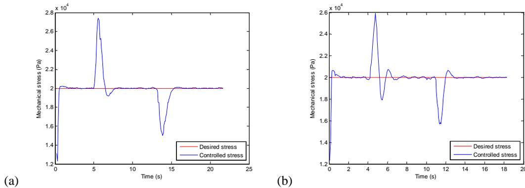
Figure 6. Disturbances at: (a) Fuzzy controller PD + I and (b) PID Controller.
