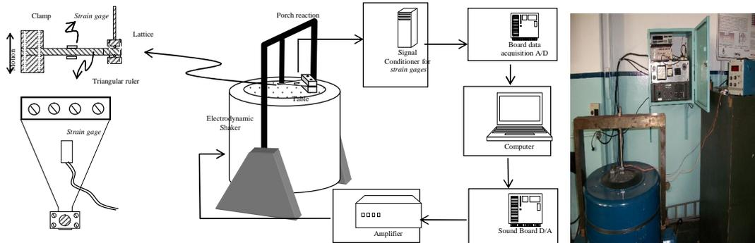
Figure 4. Scheme of control system and photo of the prototype tested.
