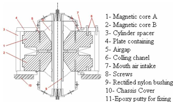
Figure 1. Parts of a generic electrodynamic shaker.
