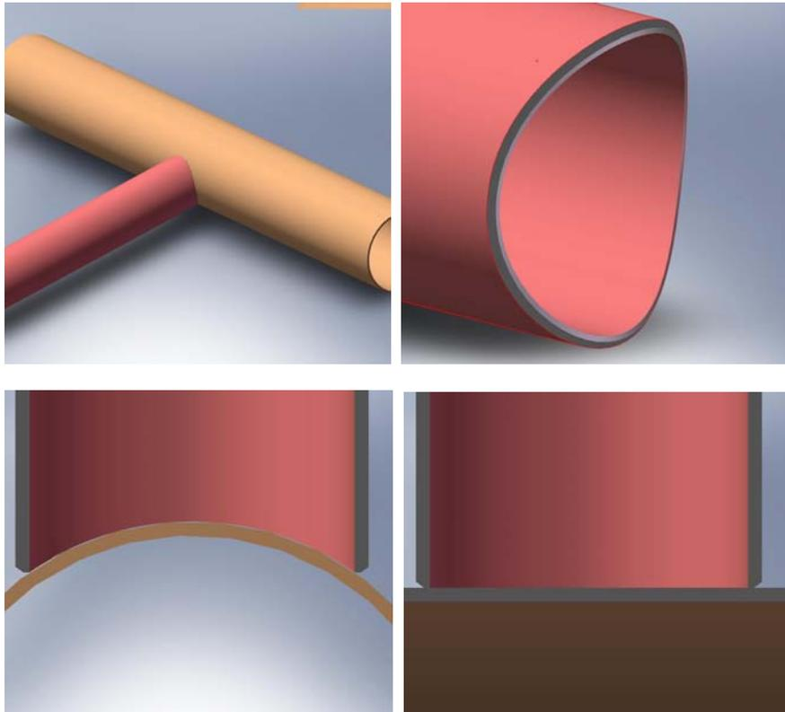
Figure 12: T junction, very common on hot tapping procedures, with complex trajectories, and variable junction to be welded, with almost flat groove at  $0^\circ$  and  $180^\circ$ .
