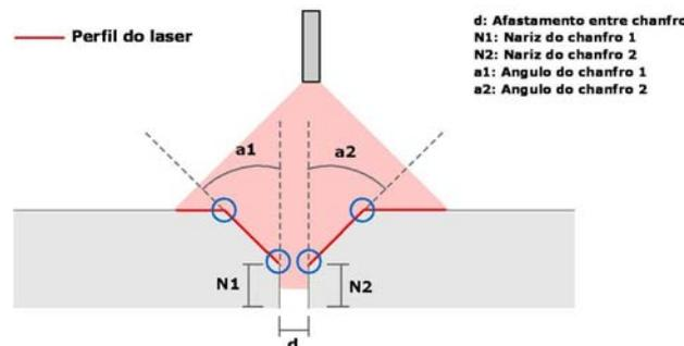
Fig. 6: Features extracted from the groove.
