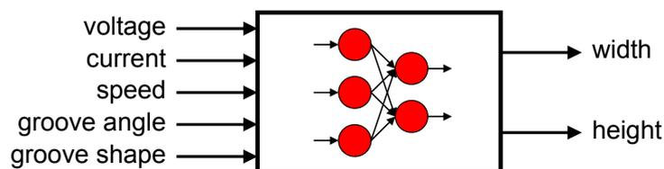
Figure 13. Welding process model using neural networks.
