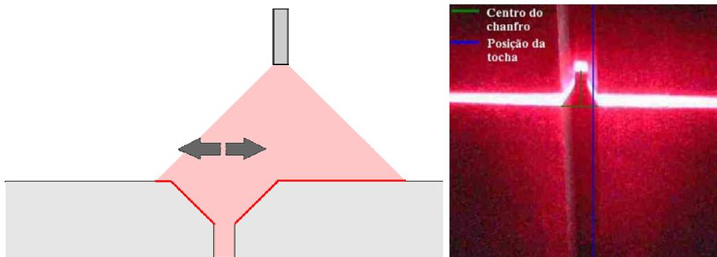
Figure 7: Trajectory deviations detection.
