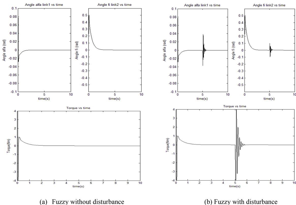
Figure 6. System with fuzzy controller optimized by ANFIS.
