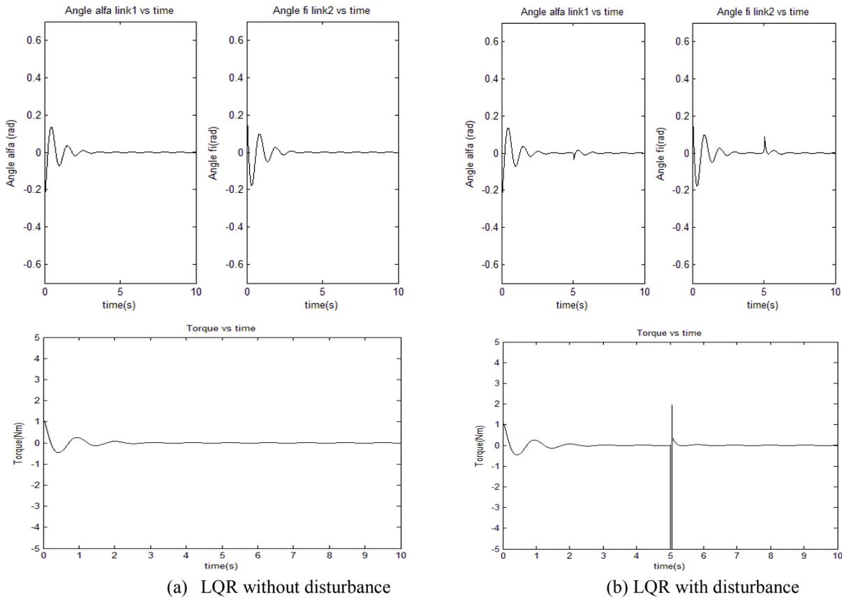
Figure 4. System controlled by LQR.
