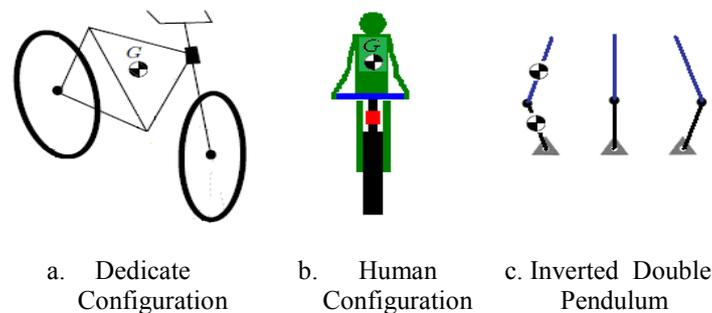
Figure 2. Model Approximation of Robot Cyclist.
