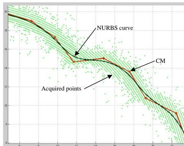
Figure 3. Example of a NURBS curve obtained from initial CM.
