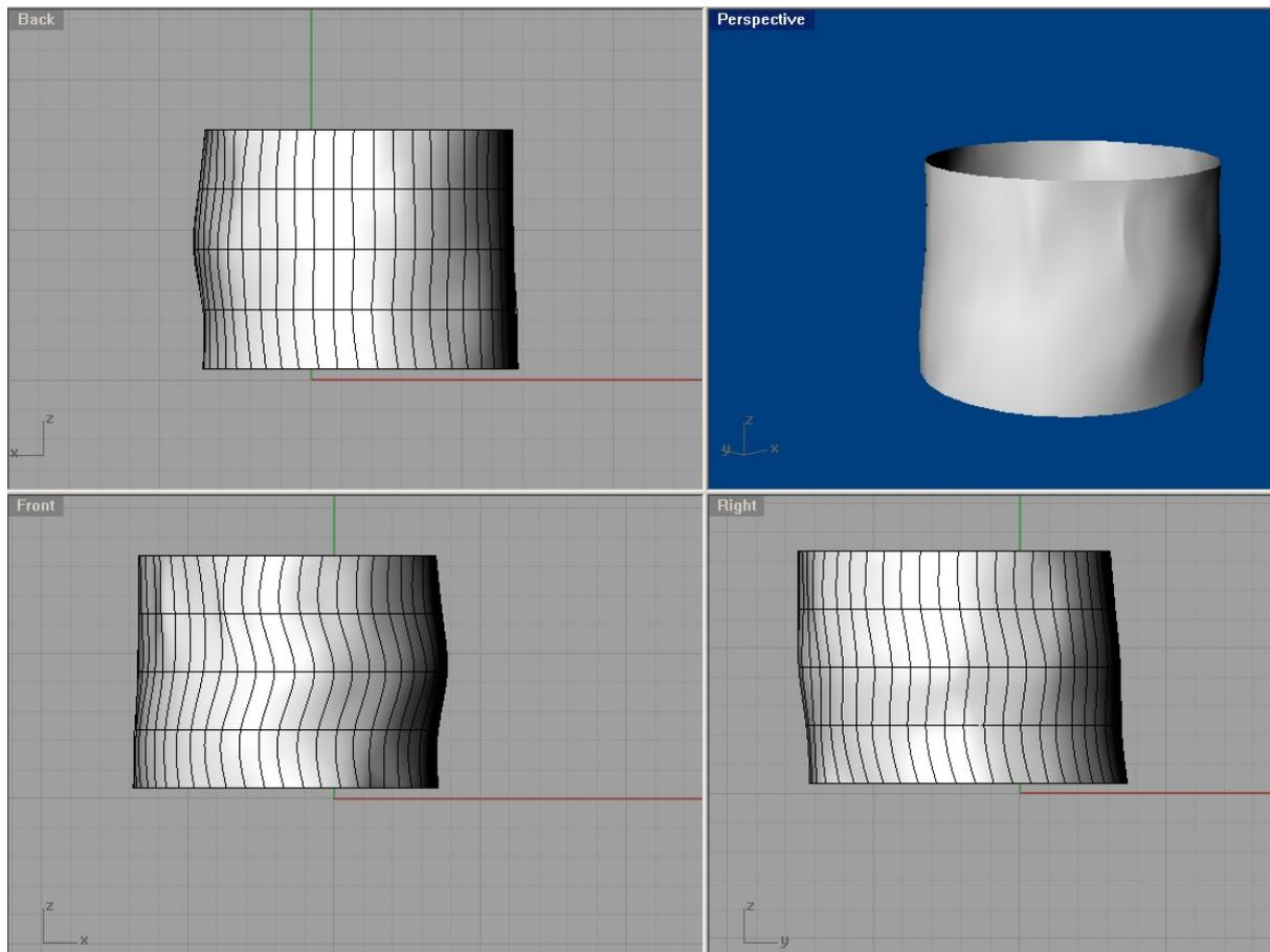
Figure 8. Rendered surface from five slices by using the proposed methodology.
