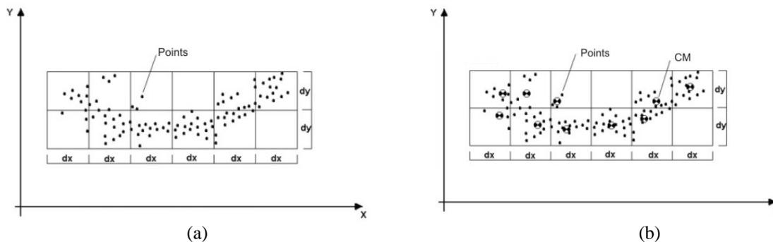
Figure 1. Method for reducing the acquired points. a) The acquired points and the regions; b) Regions and its center of mass.
