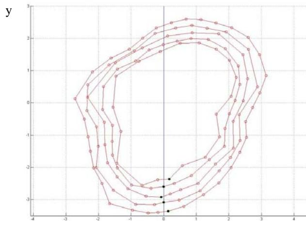
Figure 4. Selecting process for numbering the CM in order to draw the NURBS curve.
