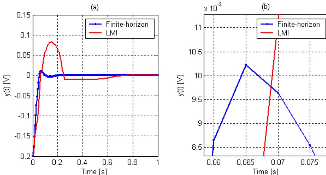
Figure 5. (a) Comparison of the presented solutions:  $K_{real} = 0.90K_{nominal}$  without robust treatment. (b) Constraint violation detail.
