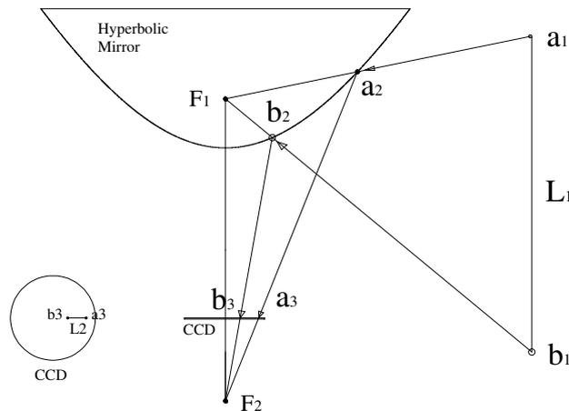
Figure 6. Projection of a straight line on the camera CCD with a hyperbolic mirror
