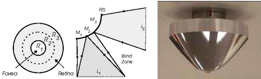
Figure 1. A triple lobed mirror (Gaspar et al., 2002)
