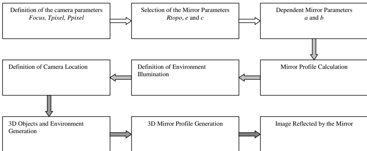
Figure 10. Block diagram showing the simulation process
