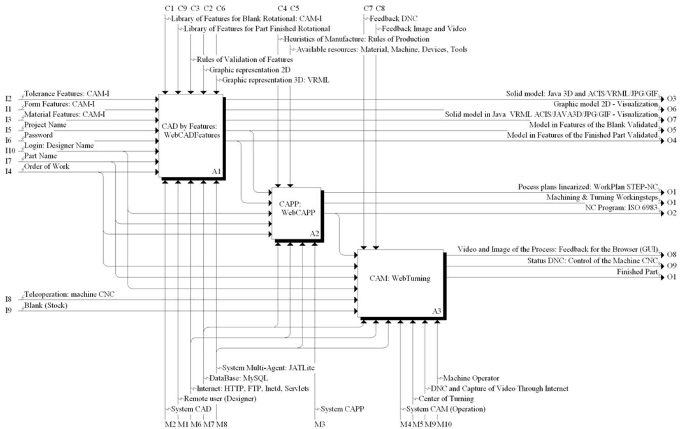
Figure 1. WebMachining: IDEF0 Model ([http://webmachining.alvarestech.com/idef0/report\\_idef0/index.html](http://webmachining.alvarestech.com/idef0/report_idef0/index.html)).
