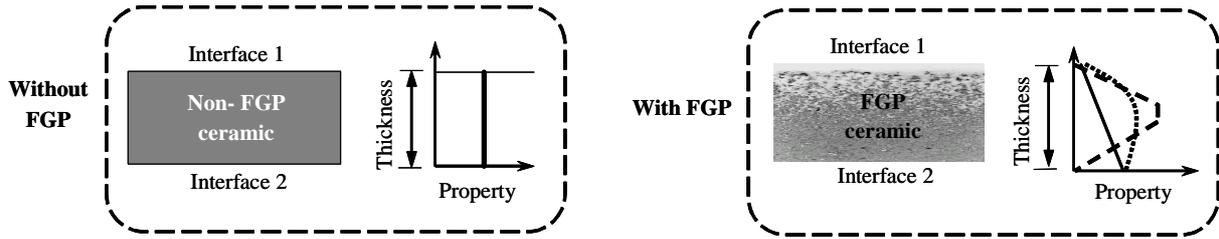
Figure 1. Sketch of a traditional (non-FGP) piezoelectric ceramic and of a FGP piezoceramic disk
