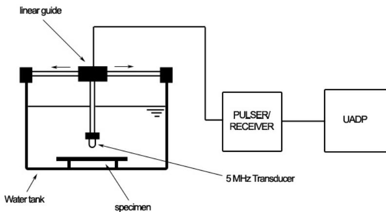
Figure 9. Experimental Setup
