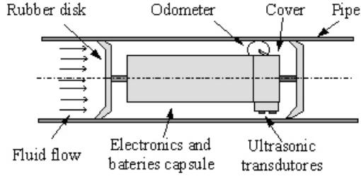
Figure 1. A pig inside a pipeline
