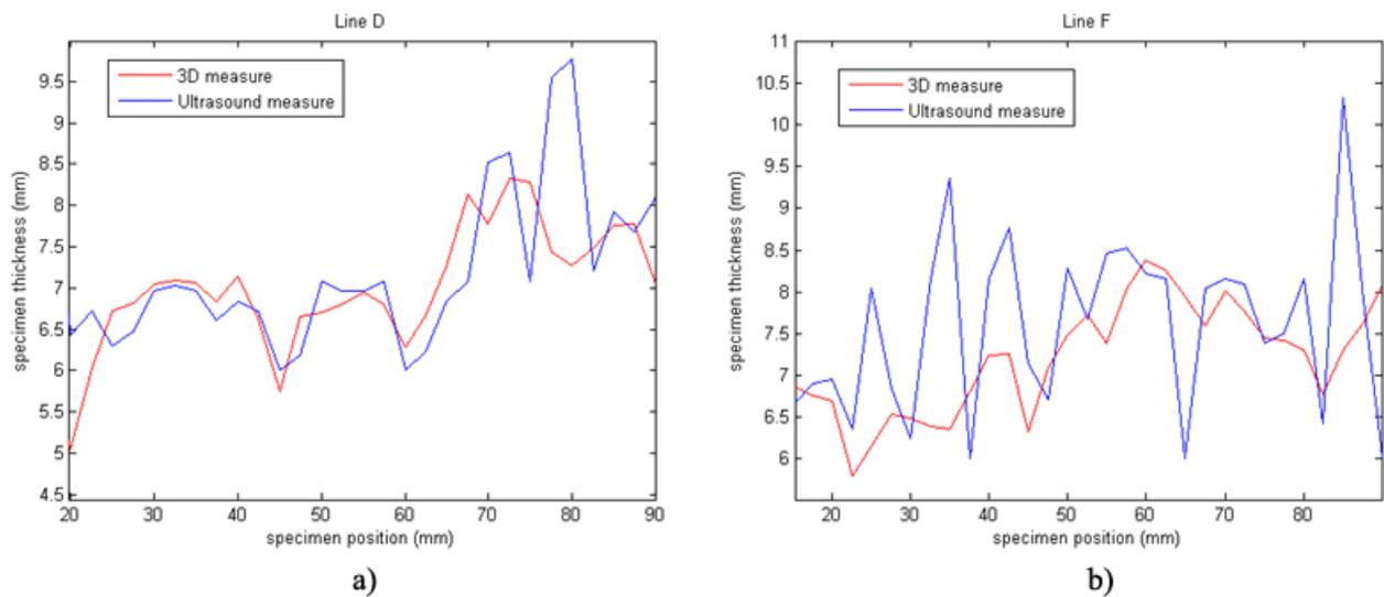
Figure 12. Thickness measure with 3D machine and ultrasound of: (a) Line D and; (b) Line F of the specimen
