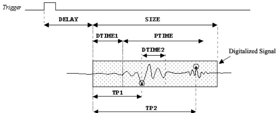
Figure 6. Peak detector programmable parameters
