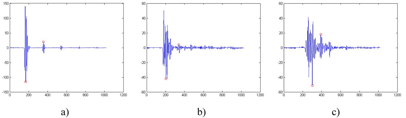
Figure 10. (a) Signal with good S/N ratio, resulting in a good detection of the TOAs; (b) and (c) Weak signals, resulting in unreliable TOA estimations
