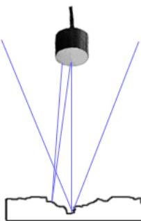
Figure 7. Ultrasound signal being dispersed in the corroded area
