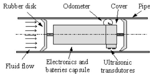
Figure 1. A pig inside a pipeline
