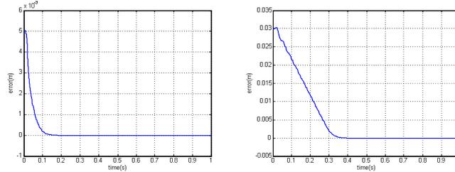
Figure 9 - Position error: short and long trajectories
