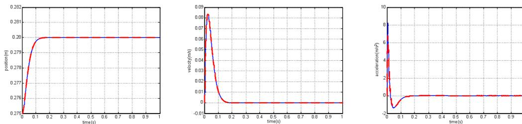
Figure 12 - Comparison between position, velocity and acceleration (blue lines) and the corresponding observer estimated values (red dashed line) – short trajectory
