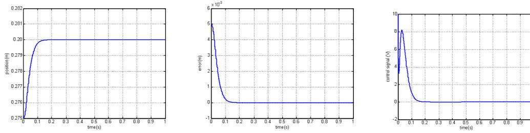
Figure 3 – Short Trajectory: position, error, and control signal
