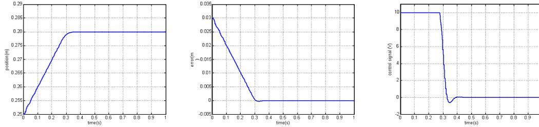
Figure 4 – Long trajectory: position, error, and control signal
