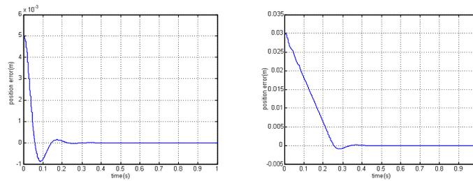
Figure 19 - Position error: short and long trajectories
