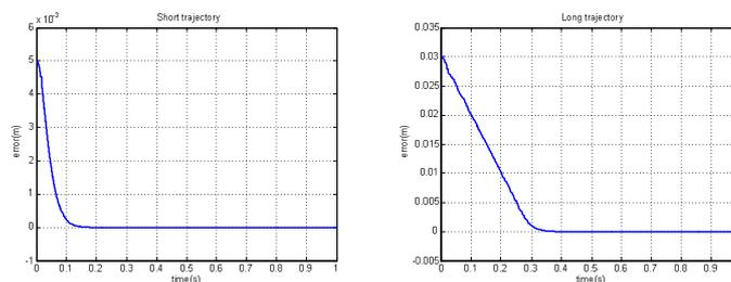
Figure 6 – Position error: short and long trajectories
