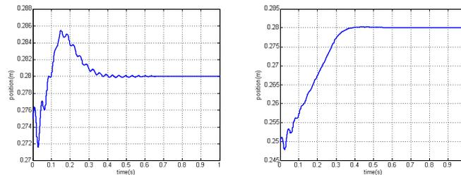
Figure 23 - Position with a filter of 30 rad/s
