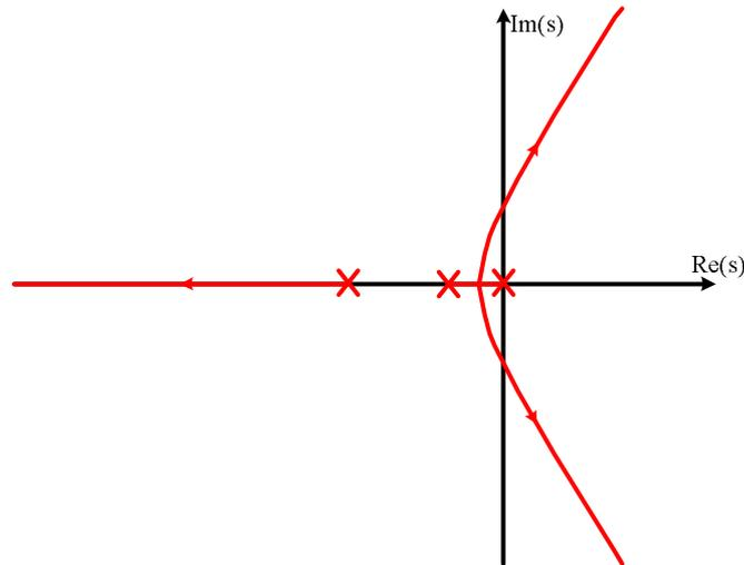
Figure 2. Root locus with the poles at new location
