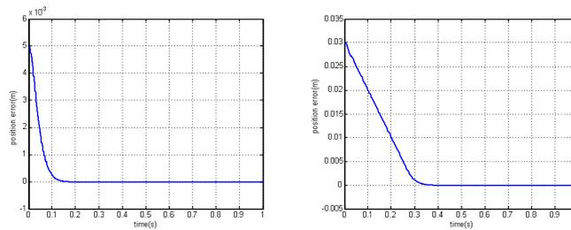
Figure 14 - Position error: short and long trajectories
