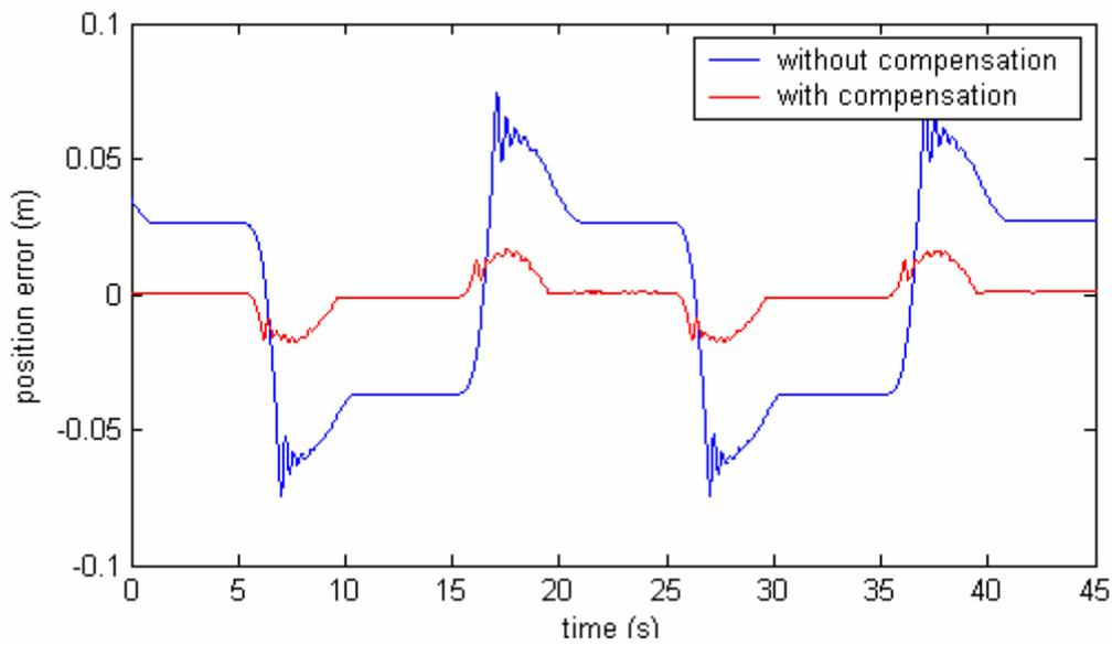
Figure 7. Position error to polynomial trajectory
