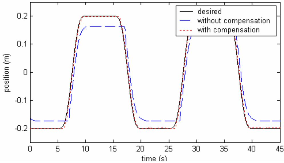
Figure 5. Experimental results to polynomial trajectory tracking
