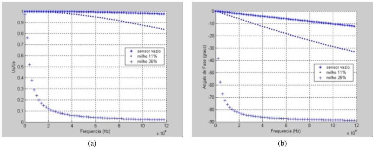
Figure 5. Frequency response simulation for  $R_1$  equal to  $10k\Omega$ : (a) Amplitude ratio  $U_s/U_e$  (b) phase angle  $U_e/U_s$
