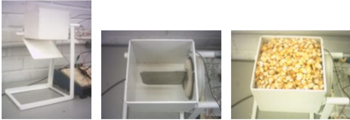
Figure 1. Moisture Sensor final mechanical conception(Lagares and Sousa, 2006)
