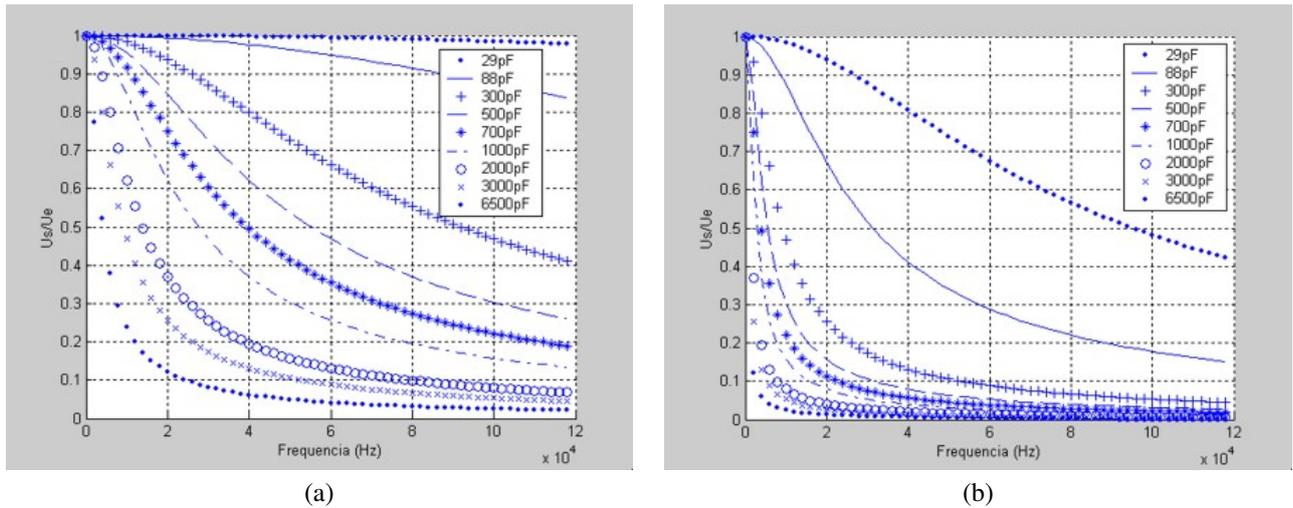
Figure 4. Amplitude ratio  $U_s/U_e$  to: 29, 88, 300, 500, 700, 1000, 2000, 3000 e 6500 pF ( $R_2$  constant equal  $1G\Omega$ ): (a)  $R_1 = 10k\Omega$  (b)  $R_1 = 100k\Omega$
