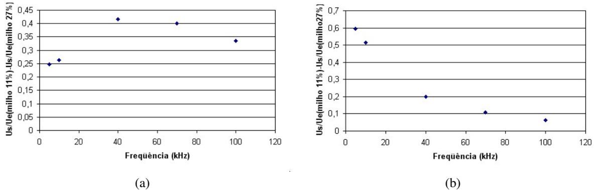
Figure 8. Experimental determination of difference between  $U_s/U_e$  for dry corn (11%) and  $U_s/U_e$  for moist corn (27%): (a)  $R_1$  equal to 10kΩ (b)  $R_1$  equal to 100kΩ
