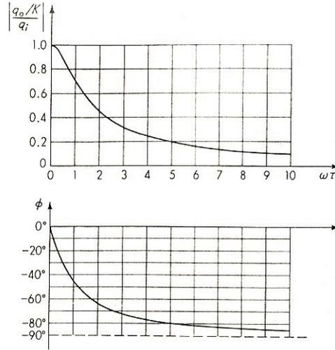
Figure 3. Nondimensional representation of eq. 8 and 9 (Doebelin, 1990)
