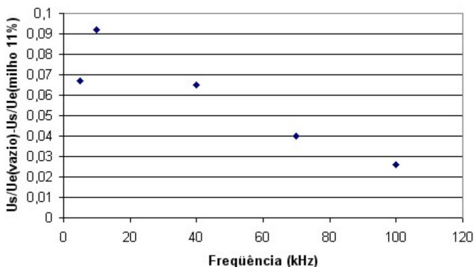
Figure 9. Difference between  $U_s/U_e$  for empty sensor and  $U_s/U_e$  for dry corn (11%)
