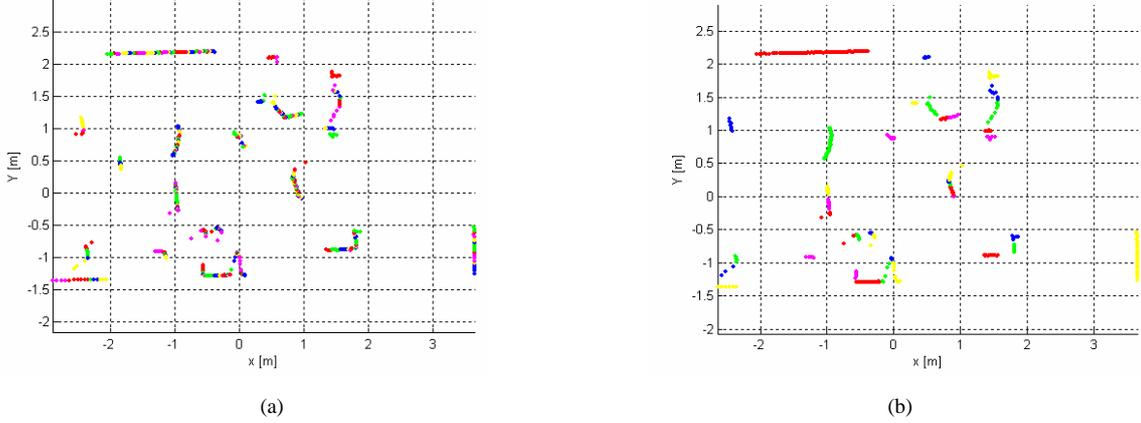
Figure 1. A scan image from two SICK LMS 200 laser range finders that is over segmented (a) and the same scan image after segment integration (b). Each segment is represented by a different color.
