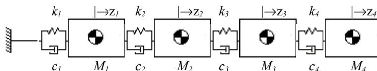
Figure 1 – Physical representation of the link.
