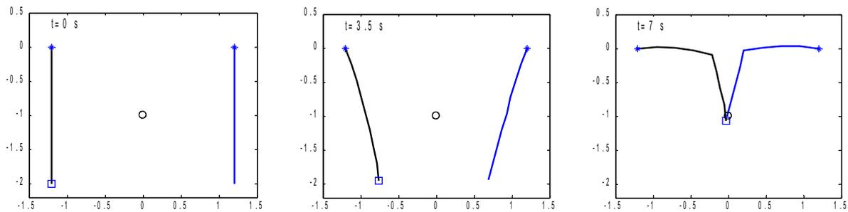
Figure 5. Robot movement given by optimal torque profile.
