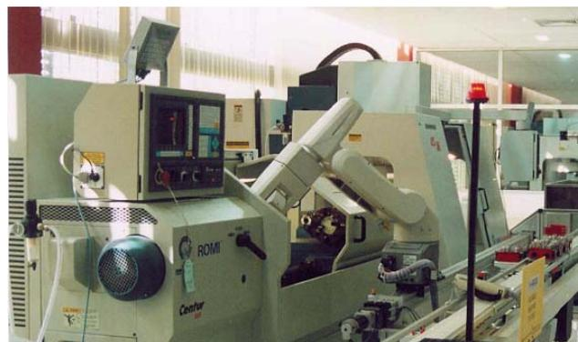
Figure 2 –Machining cell.
