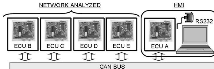
Figure 5. Schematic of CAN network for the experiment
