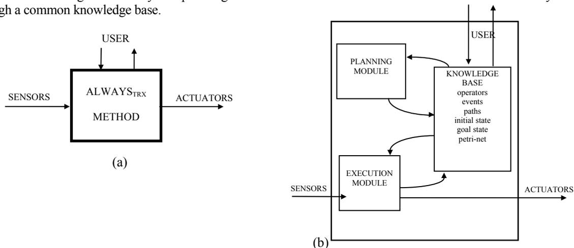
Figure 1. (a) ALWAYS<sub>TRX</sub> method in the context "see, think, act"; (b) ALWAYS<sub>TRX</sub> method's internal architecture.
