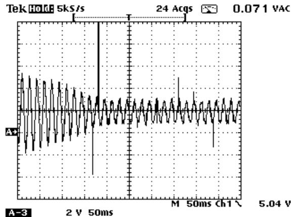
Figure 3. Phase current following a sudden change of speed.
