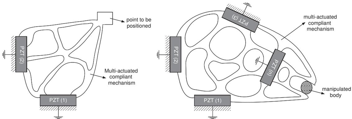
Figure 1. Concept of a multi-actuated flextensional piezoelectric devices. a) *XY* nanopositioner; b) Piezoceramics are responsible for *XY* displacements, rotation, and open/close movement of jaw.
