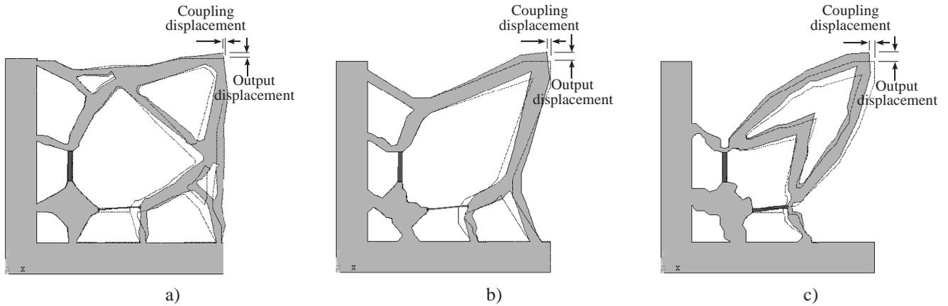
Figure 8. Displacement of XY nanopositioner obtained by FEM. a) XY05b, b) XY05, and c) XY08.
