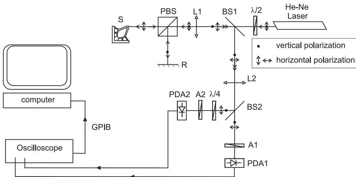
Figure 10. Experimental setup of Michelson-type quadrature interferometer. L1, L2 - convergent lens; BS1, BS2 - beam splitter; PBS - polarizing beam splitter; R - reference mirror; S - sample;  $\lambda/2$  - half-wave plate;  $\lambda/4$  - quarter-wave plate at 45°; A1, A2 - polarizing at 45°; PDA1, PDA2 - amplified photo-diode, GPIB - communication protocol.
