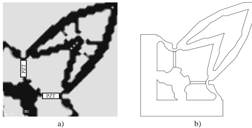
Figure 7. a) Topology optimization result for actuator XY08; b) Corresponding interpretation (CAD design).
