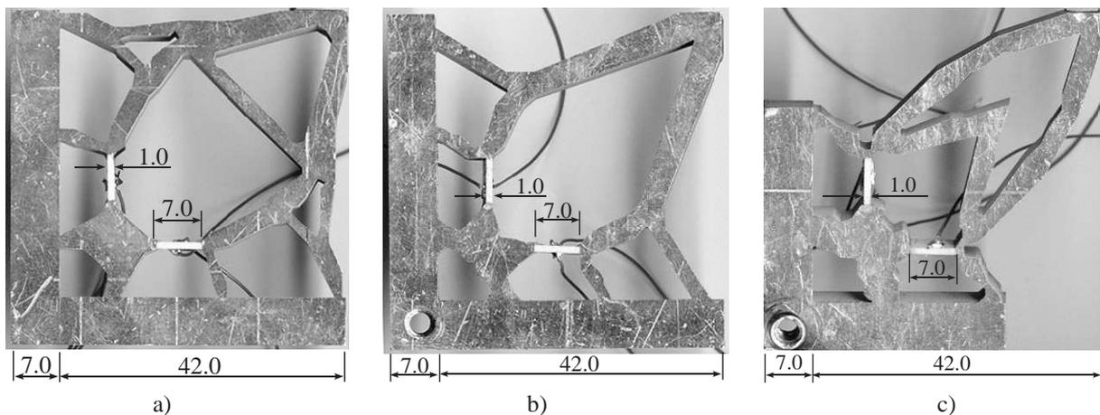
Figure 2. *XY* nanopositioner prototypes (unit mm); a) XY05b, b) XY05, and c) XY08.
