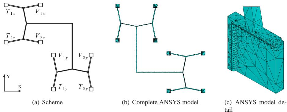
Figure 3. XY micropositioner – Scheme and ANSYS model
