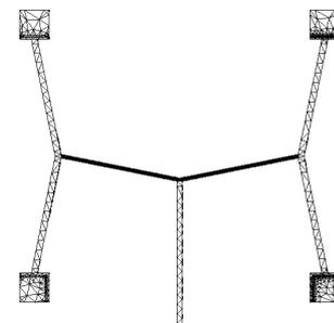
Figure 6. XY micropositioner with two materials (white: nickel; black: copper)
