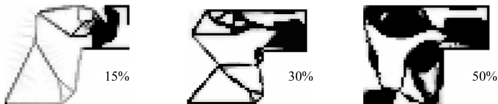
Figure 9. Influence of the material volume constraint in the final topology.
