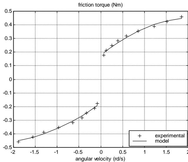
Fig. 2 Friction torque: experimental and model.
