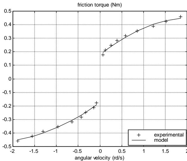
Fig. 2 Friction torque: experimental and model.
