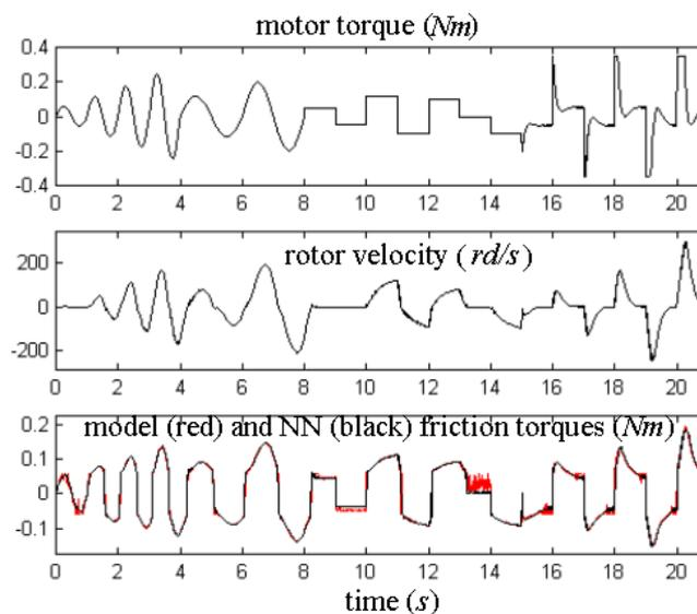
Fig. 5. Motor torque, rotor velocity and friction torque.
