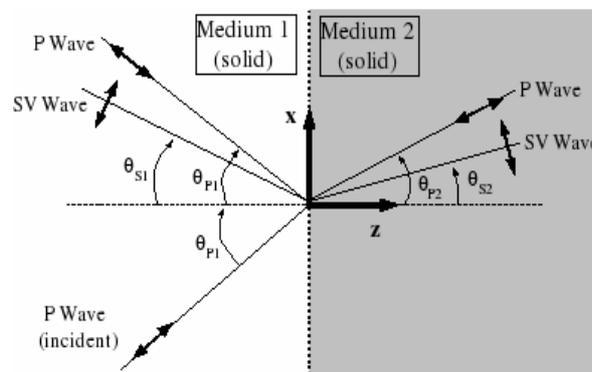
Figure 1. Longitudinal wave impinges a solid-solid interface.
