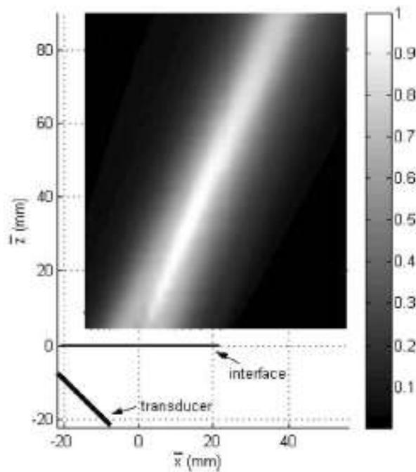
Figure 6. Simulated acoustic field through an interface
