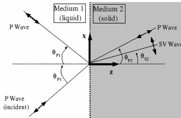
Figure 2. Longitudinal wave impinges on the interface between a non-viscous liquid and a solid.
