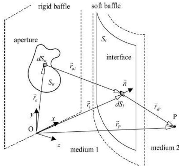
Figure 5. Geometry used to calculate the field produced by an arbitrary source through an arbitrary interface
