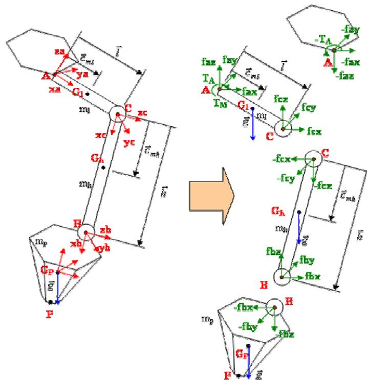
Figure 2. Hexa's free body diagram. For simplicity, the notation was changed:  $Ps_j = A$ ,  $Pi_j = B$ ,  $Pa_j = C$ ,  $Pc = P$ .  $G$  indicates the gravity centers points (which have their relative position measured by  $c_{mh}$  and  $c_{ml}$  for both types of rods);  $\bar{g}$  the gravity,  $m$  the mass,  $T$  the torques. External forces are not outlined.
