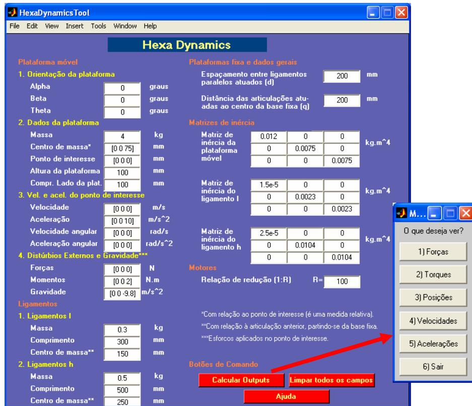
Figure 3. Dynamics Tool developed using Matlab. There are a few outputs that the user can request, such as forces, torques, velocities, accelerations.
