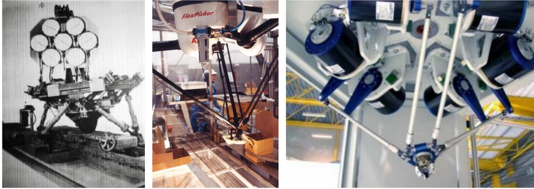
Figure 1. From left to right: Gough's Platform; ABB FlexPicker™ (Delta Architecture); Hexa from IWF
