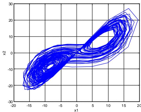
Figure 1: The  $x_1x_2$  phase plan of Lorenz system.
