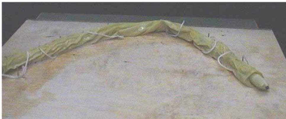
Figure 3: A balloon deployed in a latex 'colon'.
