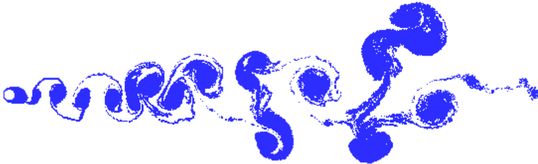
Figure 3. Position of the discrete vortices in the wake at t_f = 50.00 for an isolated circular cylinder ( Re = 1.0 \times 10^5 ).
