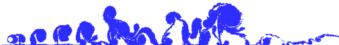
Figure 7. Position of the vortices in the wake at t_f = 50.00 for a circular cylinder in moving ground ( Case II ; h/d = 0.45 ; Re = 1.0 \times 10^5 ).
