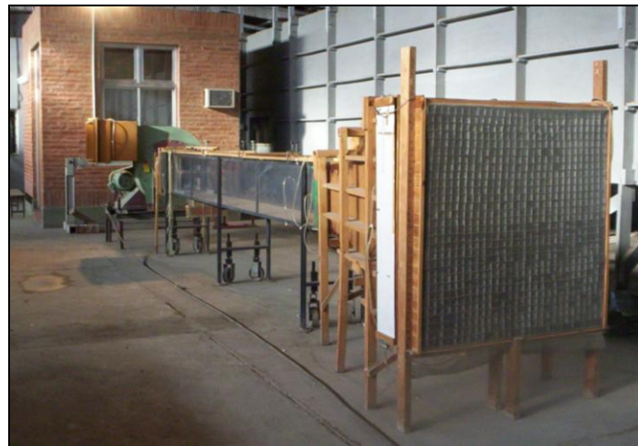
Figure 1. The wind tunnel (TV2) of the Universidad Nacional del Nordeste
