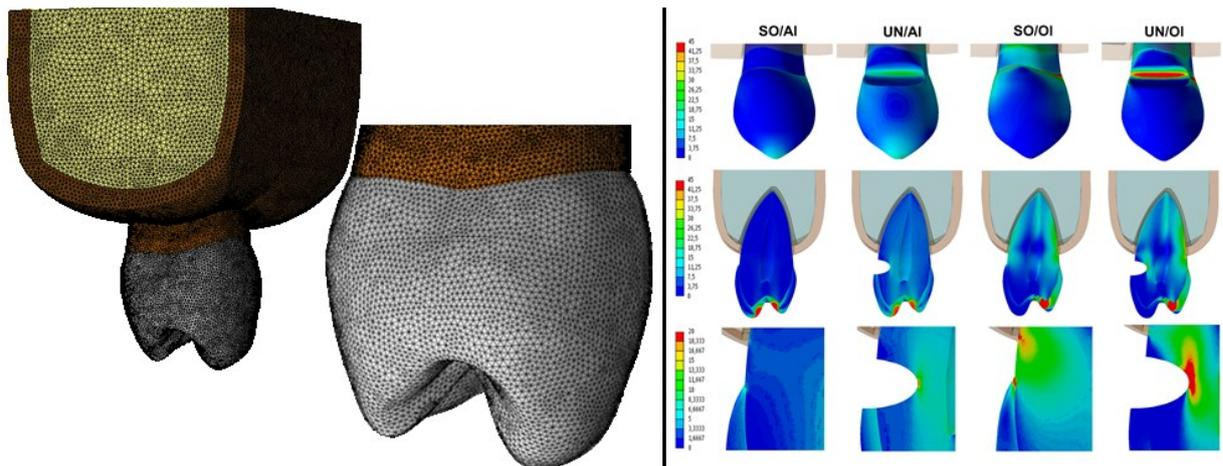
Figure 1. A. Mesh of the structures. B. Stress distribution by von Mises stress for Sound tooth (SO) and Unrestored NCCL (UN) according to the loading condition: AI- Axial loading; and OI- Oblique loading.
