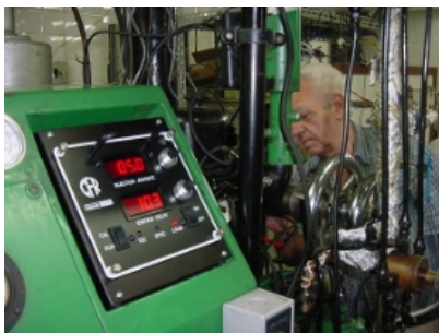
Figure 1. Engine ignition delay data acquisition system
