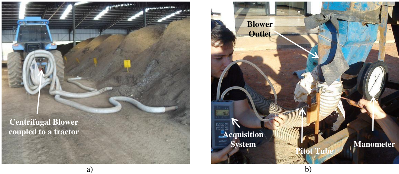
Figure 1 – Aeration in organic compost piles a) Blower coupled to a tractor and organic compost piles; b) Experiment to determine the mechanical characteristics of the blower.
