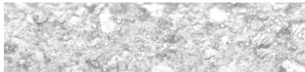
Figure 7: Typical image obtained from the Shadow Sizer system, where only the droplets deposited on the pipe wall can be characterised.
