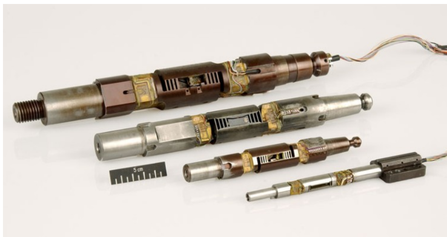
Figure 5. Some examples of sting balances manufactured by ONERA (ONERA, 2004).
