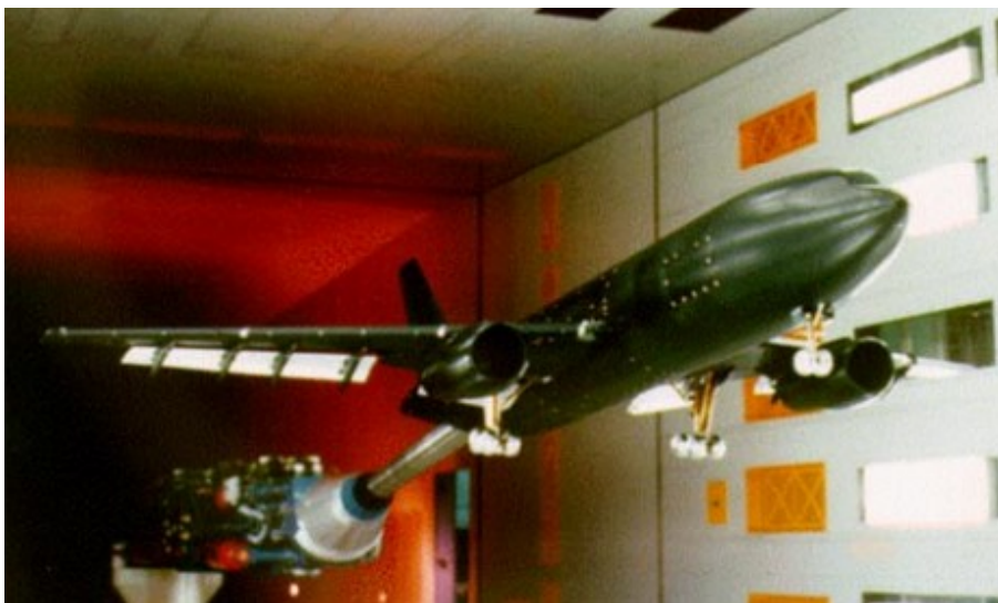
Figure 3. An Airbus model mounted on a tail sting in the Deutsch-Niederbindiseher Windkanal tunnel (Ewald, 2000).
