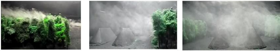
Figure 2. Flow visualization around the WTGB1 and mineral piles.
