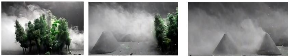
Figure 4. Flow visualization around the WTGB3 and mineral piles.
