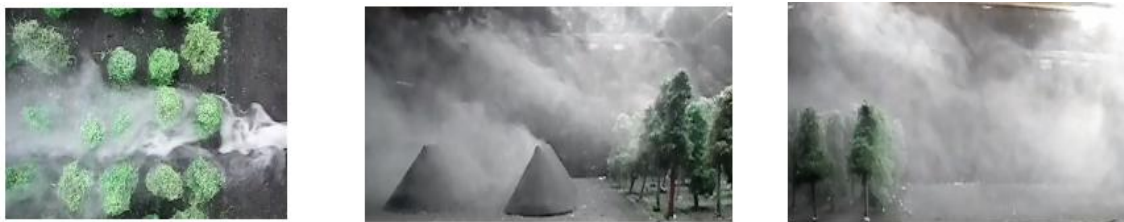
Figure 3. Flow visualization around the WTGB2 and mineral piles.
