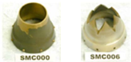
Figure 1. Nozzle geometries studied by Bridges and Brown (2004).
