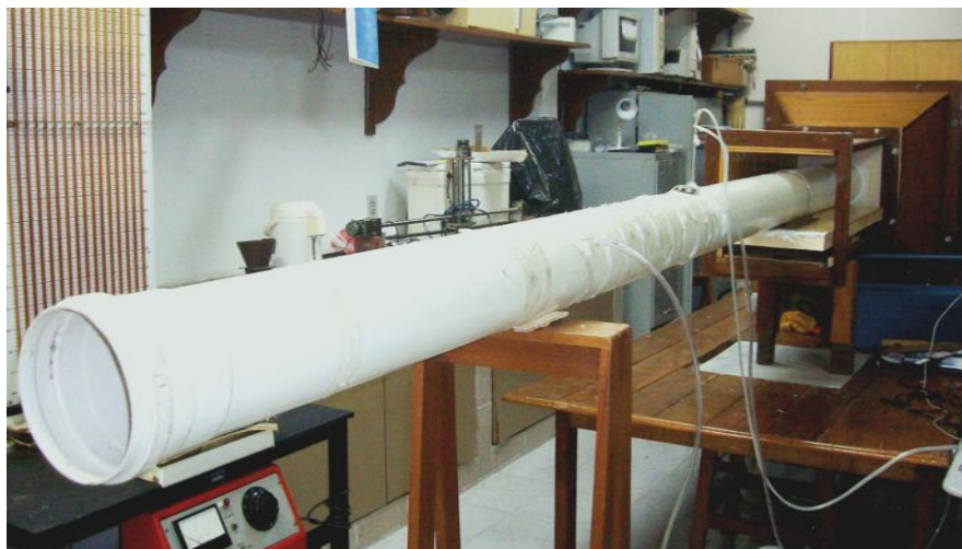
Figure 2. View of the PVC pipe coupled to a wind tunnel.
