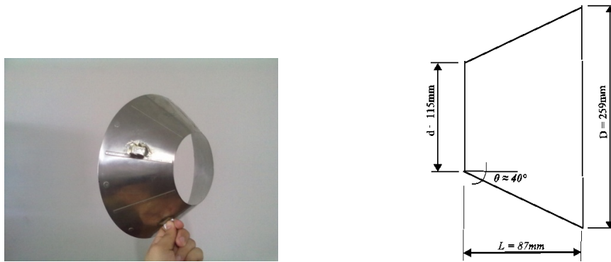
Figure 1. Diffuser and its dimensions and used in the experiment
