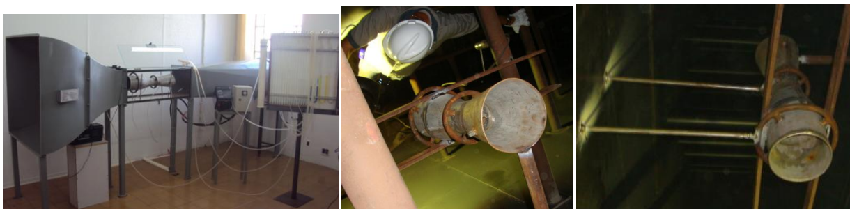
Figure 5. Venturi Tube – Calibration and Installation
