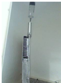
Figure 2. Charging of the working fluid.
